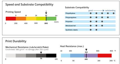
Videojet evaluation of observed performances of the Standard Ribbon with optimized printer setting and receptors.
