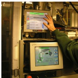
Epley investigated further and ran across information in an industry trade publication about Videojet's DataFlex printer. It caught his eye because it could do both continuous and intermittent printing. Utz uses both formats for flexible packaging, while intermittent printing is typically used for canister coding.
