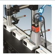
While ensuring that the printer has the right data is an essential starting point for code assurance, it does not fully guarantee each individual product will have the necessary code information when it leaves your packaging line. For various reasons, the code may be missing, applied in the wrong place or most commonly, become illegible over the course of the production run.
