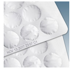
Thermal inkjet code on blister foil
