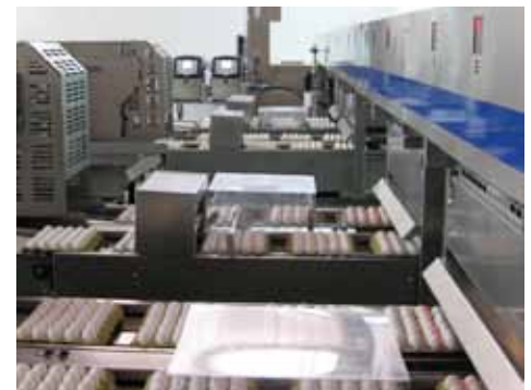
CIJ printers installed on grader
