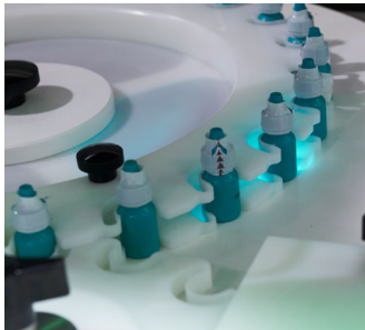
Star wheel transport for positive bottle control during marking
