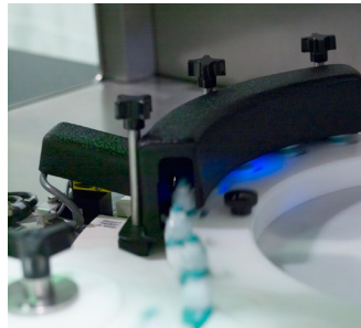
Bottles being marked on bottom; laser shield shown in black
