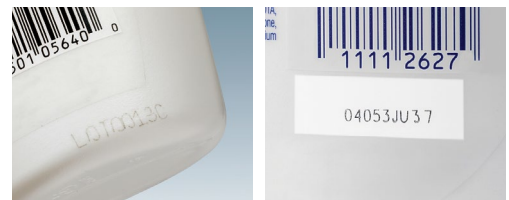
Illegible and misplaced code
