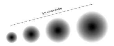
The spot size is determined by the combination of marking head aperture (6, 10, 12mm) and lens. The laser 'power' is distributed over the spot's area which results in a certain 'power density' for a given laser power and the spot size. It is important to understand that the spot's area increases with the square of its diameter. Consequently, if the spot size is increased by a factor of two, the power density is reduced by a factor of 4 (down to a quarter).
