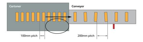
**Picture above:** Best mounting position is inside the cartoner (oval circle) as the product to be marked is guided. In contrast, marking on the conveyor belt (although seems the most obvious) induces the risk of product movement and hence possibility of lower mark quality.
