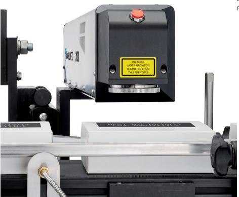
Mechanical options typically refer to separating the beam delivery from the marking head. This can be achieved via beam extensions or beam turning. Beam Turning Units (BTUs), or so called 'optical plumbing', allow for clean placement of a scan head (Marking head) inside a piece of equipment like a cartoner, flow wrapper, bagger, etc. while mounting the laser body somewhere out of the way from hazards like lift trucks, pallet jacks, careless operators, and so on.
