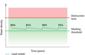
To compensate the loss of power and assure that even after 5-7 years of operation the laser is still fully capable of achieving the desired performance, all initial marking tests should be done with less than 100% output power. This allows additional power to be available for adjustment over time.
