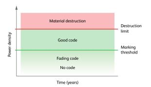
Power density below the marking threshold may result in weak or faded codes, however, increasing the power density too much could exceed the second threshold (destruction limit) and potentially damage the material. Only if the right amount of power density is applied, will consistent, high contrast codes be achieved.
