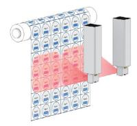
**Two** lasers using 340mm wide mark window
