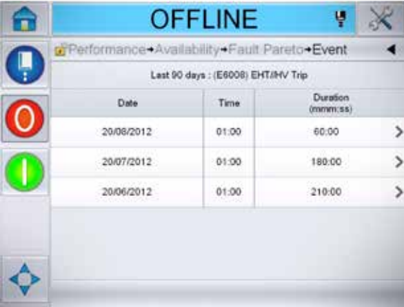
Drilling down to reveal the date, time and duration of each fault.
