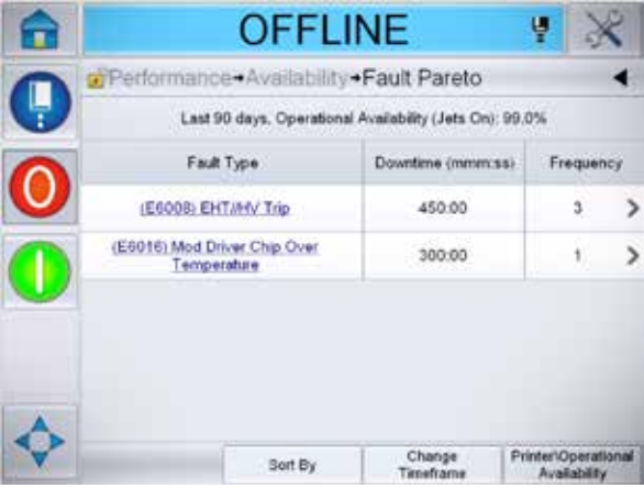
Drilling down from raw availability information to specific root causes.
