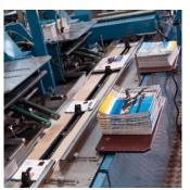
The mailing solutions industry is high volume and low margin, so quality and productivity are the main benefits sought from an addressing machine in the Graphics industry. Reduced downtime is critical; ink is required to dry instantly to provide a non-smudging solution, and the quality of the print needs to be consistent across film and all other printing products.
