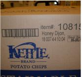
"For us, labeling means storing, printing and applying labels to each case," Manzer says. "We like to print right on the box because we can avoid wasted labels, waste from label backings and unnecessary time to apply labels."
