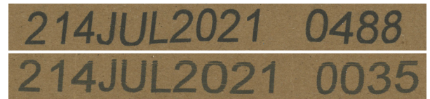
Inkjet codes on Gonnella cases from Videojet ink M533 (top) versus M512 (bottom).
