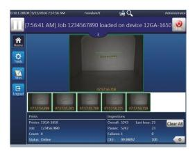
VCIS tracks key production statistics such as throughput and pass/fail rate and provides a visual display of associated trends
