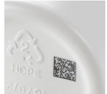
The Videojet 7810 laser system leverages Ultraviolet wavelengths to create permanent, high resolution codes on HDPE packaging
