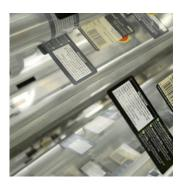
TTO is a clean, no-mess printing technology that is friendly to operators and production environment. No solvents are used and ribbon waste can be disposed of without special arrangements for hazardous substances.
