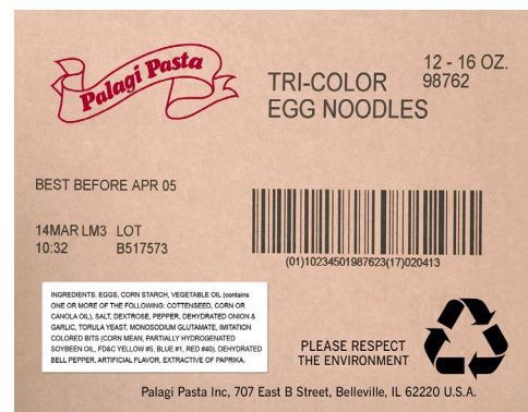
Case with pre-printed color logo and ingredients listing along with variable, on-demand printing
