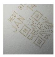
Laser marking is a process of ablation, where the laser etches the top surface of the egg. It 'bleaches' the surface of brown eggs and darkens the surface of white eggs.
