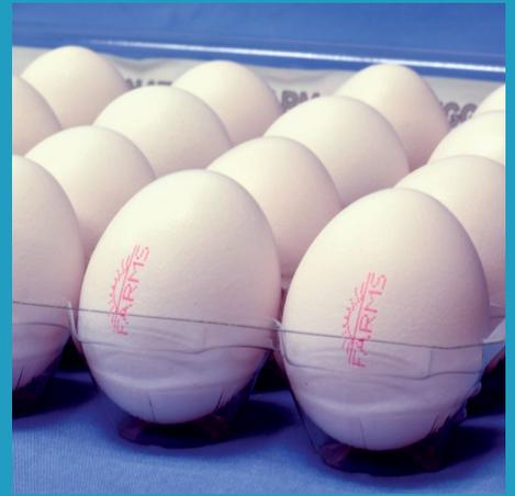
In modern high capacity grading equipment, as many as 10 eggs will pass in front of a printhead every second. Since any egg can be destined for any packing lane, it can be printed with any code.
