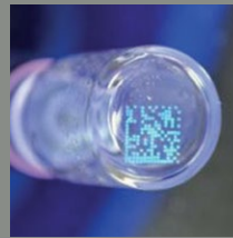
Videojet UV ink on glass vial bottom
