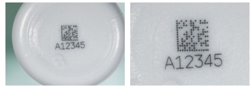
High contrast UV laser mark on HDPE bottle
