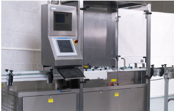
FP Developments packaging solution including Videojet UV laser installation
