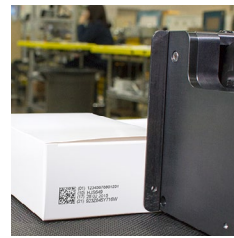
2D DataMatrix code on a coated carton
