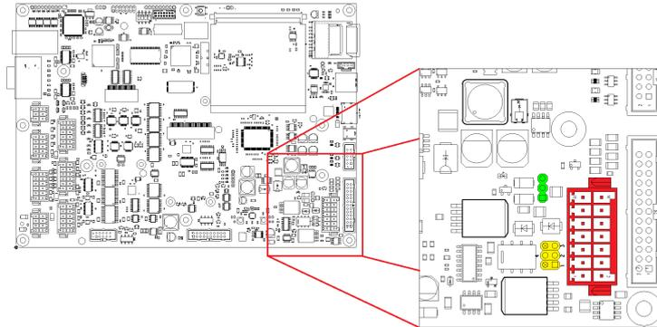
The jumpers X19 (yellow) and X20 (green) are used for configuration.
