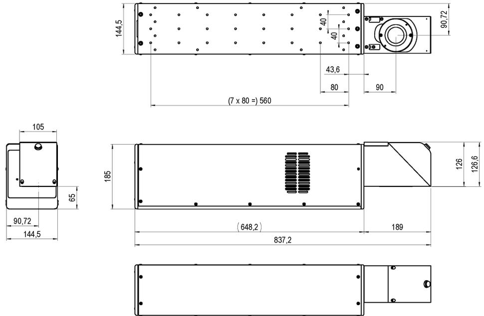
Marking Unit (Laser Head and Marking Head) Videojet 3640
