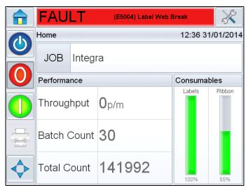
Figure 8-3: Fault Display
