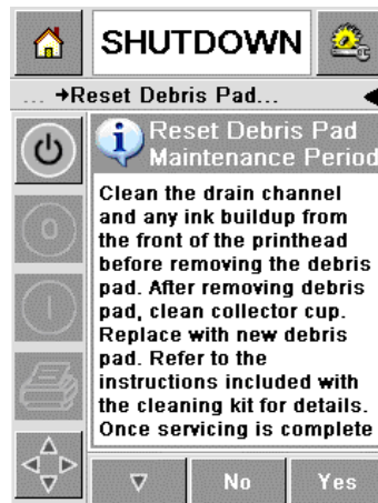
Figure 4-28: Removing the Debris Collection Pad
