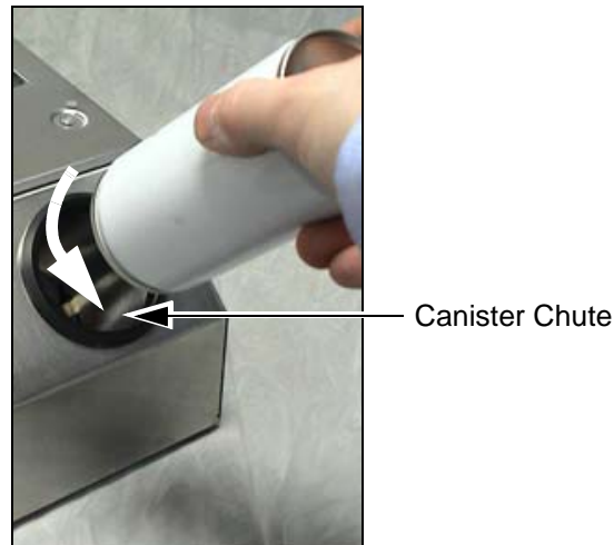
Figure 4-12: Removal of Empty Ink Canister
