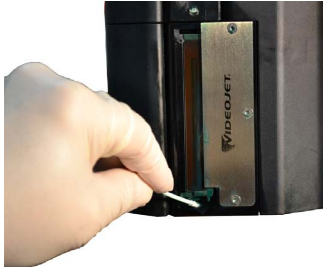
Figure 4-26: Cleaning the Collector Cup (Videojet 2351/2361)
