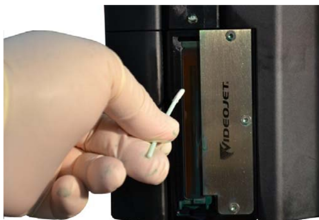
Figure 4-23: Drain Channel Cleaning (Videojet 2351/2361)
