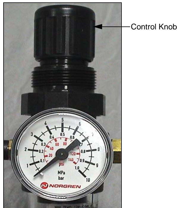
Figure 4-4: Air Regulator for Videojet 2340, 2351 and 2361
