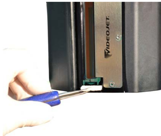
Figure 4-25: Debris Pad Removal (Videojet 2351/2361)
