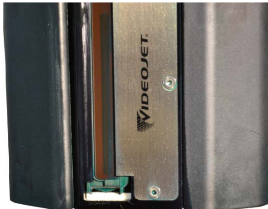
Figure 4-27: Debris Pad Inserted (Videojet 2351/2361)
