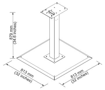
Figure A-3: Static Printer Stand
