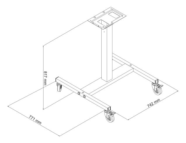
Figure A-2: Mobile Printer Stand Dimensions
