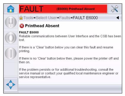
Figure 7-7: Fault Details Display
