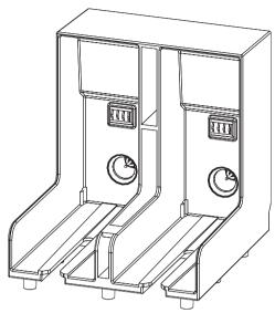
Figure 6-3: Cartridge Holder Slot
