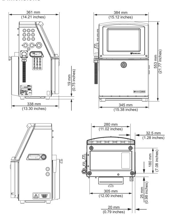
Figure A-1: Printer Dimensions
